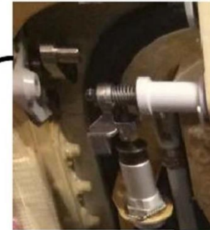
CABLE PULLED BY SLIDE RELEASE PERCUSSION MECHANISM CABLE
