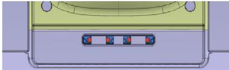
UNLOCKED BUT STILL LATCHED. (INNER HANDLE AT 47.5 DEGREES)
