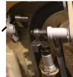
CABLE PULLED BY SLIDE RELEASE PERCUSSION MECHANISM CABLE
